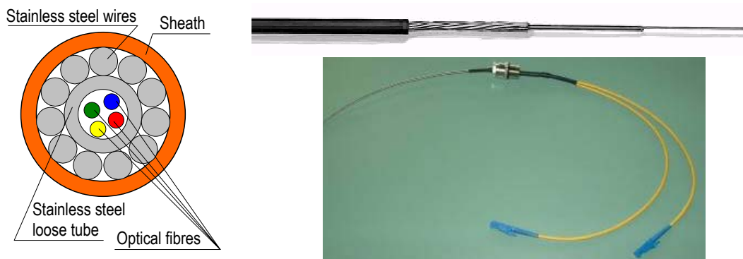
Figure 1: Extreme temperature sensing cable design and termination.
